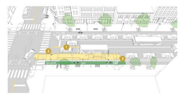
• The boarding platform must at minimum span from the front door to the rear door, and may be extended to meet capacity demands (i.e. 60 ft as per Transit Windsor comments);
